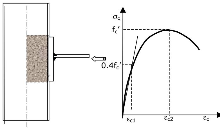
Figure 2: Infilled concrete subject to compression
