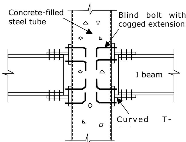
Figure 1: A typical blind-bolted T-stub connection
