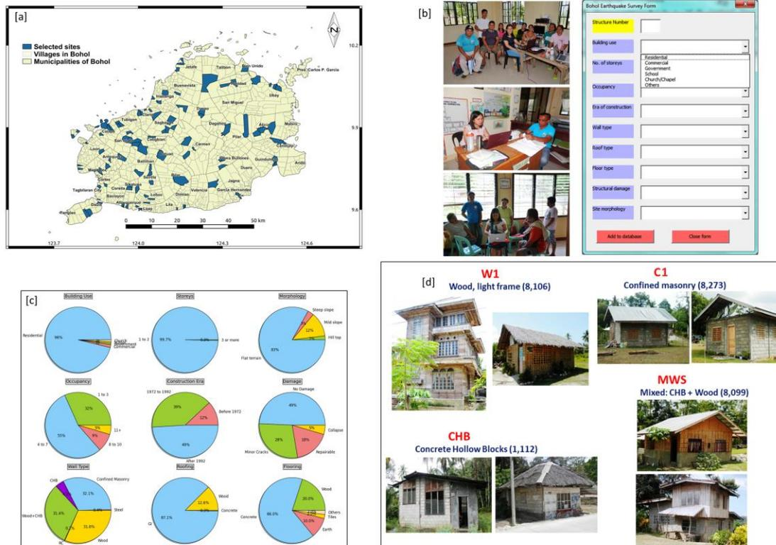
Figure 2. [a] Strategic locations of villages in Bohol where the post-event interviews were conducted; [b] Interviews with the locals & the survey form showing the structural attributes; [c] Summary of the exposure/damage database; and [d] Typical building types in the database
