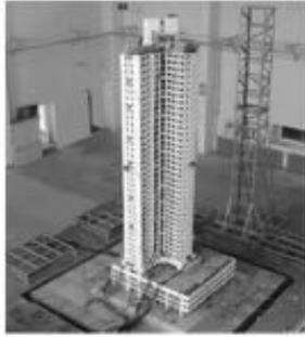
Figure 3: 1:20 Scaled test prototype
