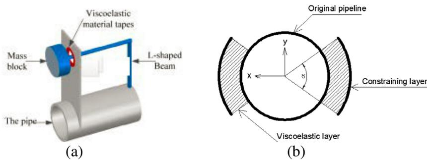
**Fig. 1.** Recently proposed methods for above-ground pipeline vibration control (a) PTMD (after Song et al. (2016)) and (b) constrained viscoelastic material (after Bi and Hao (2016b))
