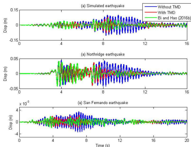
**Fig. 7.** Transverse displacement time histories at the middle of the pipeline for the uncontrolled and controlled systems
