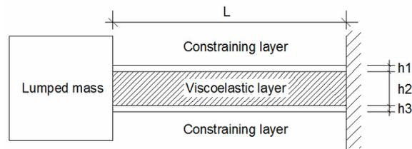
**Fig. 3.** A typical viscoelastic TMD
