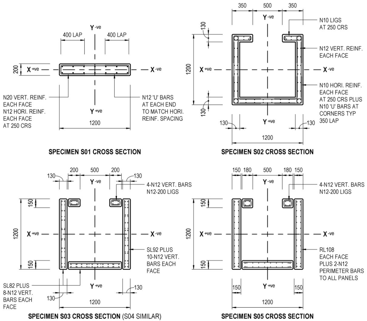
Figure 2. Wall specimen cross sections.
