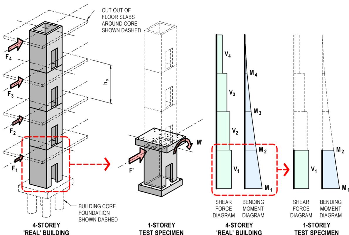
**Figure 1.** Four-storey 'real' building versus one-storey test specimen.
