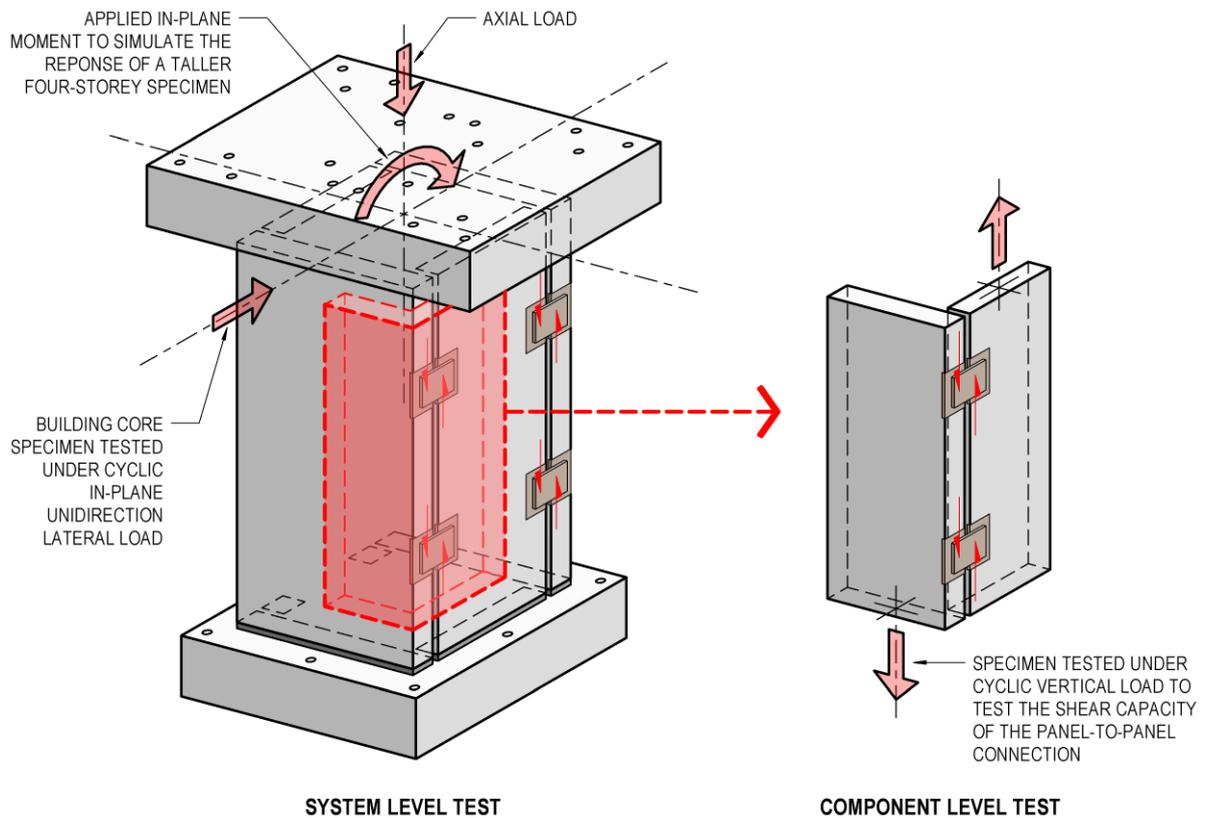
Figure 5. Precast core connection testing (Menegon et al. 2017a).
