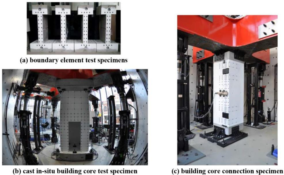
Figure 3. Test specimen photos.
