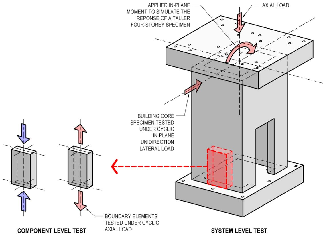
Figure 4. Boundary element prism testing.
