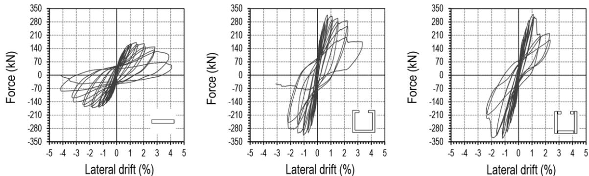
**Figure 6.** Force-displacement response for test specimens S01 (left), S02 (middle) and S05 (right).
