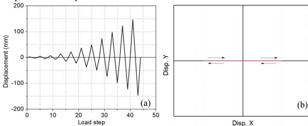
Fig. 3 (a) Uniaxial loading protocol, (b) Uniaxial loading path
