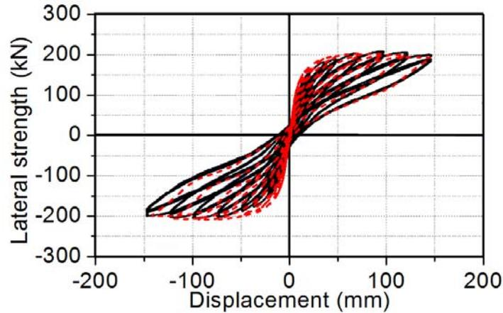
Fig. 4 Comparison of modelling and experimental results
