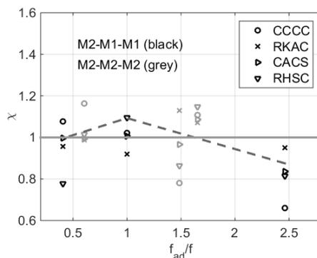
Figure 6. Acceleration amplification for three adjacent models compares to the stand-alone case
