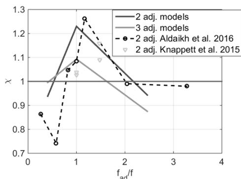
Figure 7. Amplification for two and three adjacent buildings
