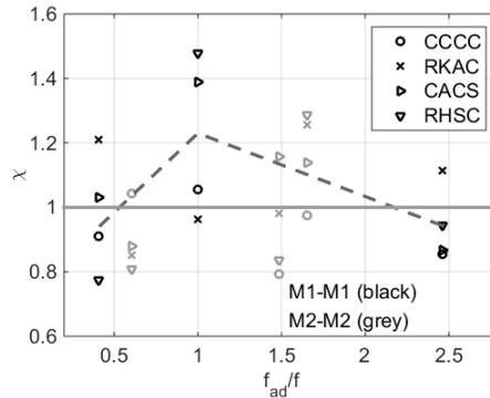
Figure 4. Acceleration amplification for two adjacent models compares to stand-alone case
