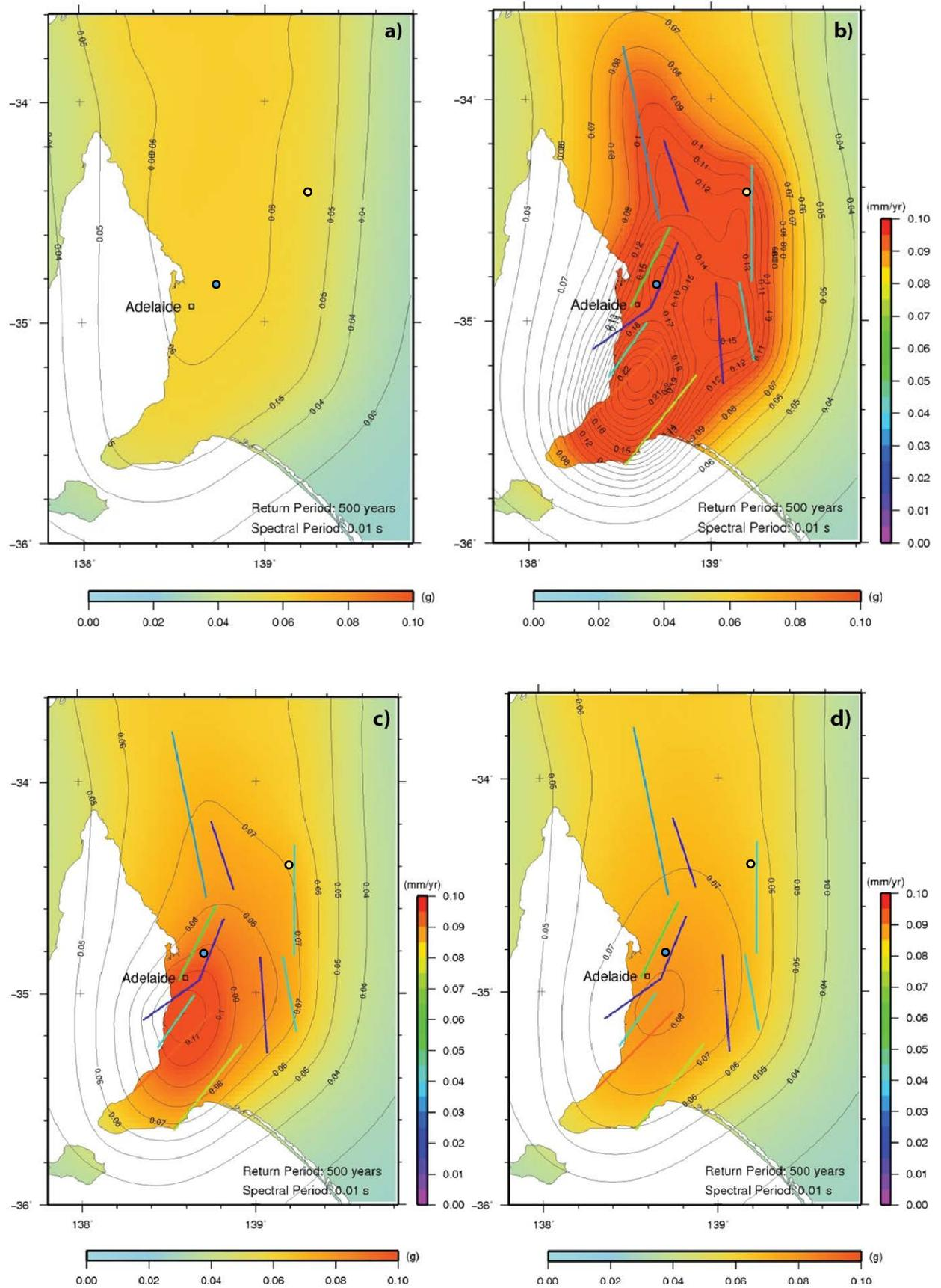
Figure 3. Comparison of 500 year return period hazard values for the Adelaide region calculated using (a) no faults, (b) G-R faults, (c) CE faults, and (d) CE faults with  $M_{\min}$  of Mw 5.5. Faults are coloured by slip rate. The blue and yellow dots mark the locations considered in Tables 1a and 1b, respectively. Note that hazard values increase significantly (20-58%) by including CE faults and up to 220% where G-R faults are used.
