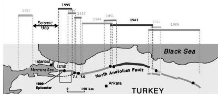
Figure 2 North Anatolian Fault and its Ruptures
