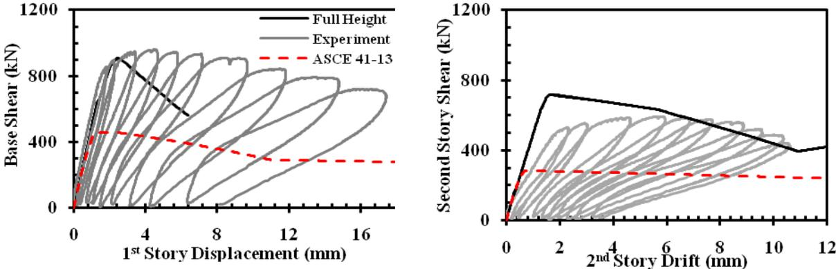
**Fig. 3 – Analysis results for test building B8**
