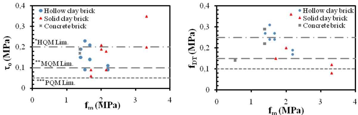
**Fig. 1 – Relationships between compressive strength with (a) shear strength and (b) diagonal tension strength** (\*: High Quality Mortar Limit, \*\*: Medium Quality Mortar Limit and \*\*\*: Poor Quality Mortar Limit)
