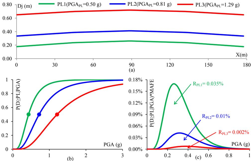
Figure 4: (a) Performance displacement profiles of the bridge in transversal direction, derived following the EMA approach, (b) Fragility curves for the selected PLs; (c) Seismic risk curves for the selected PLs.
