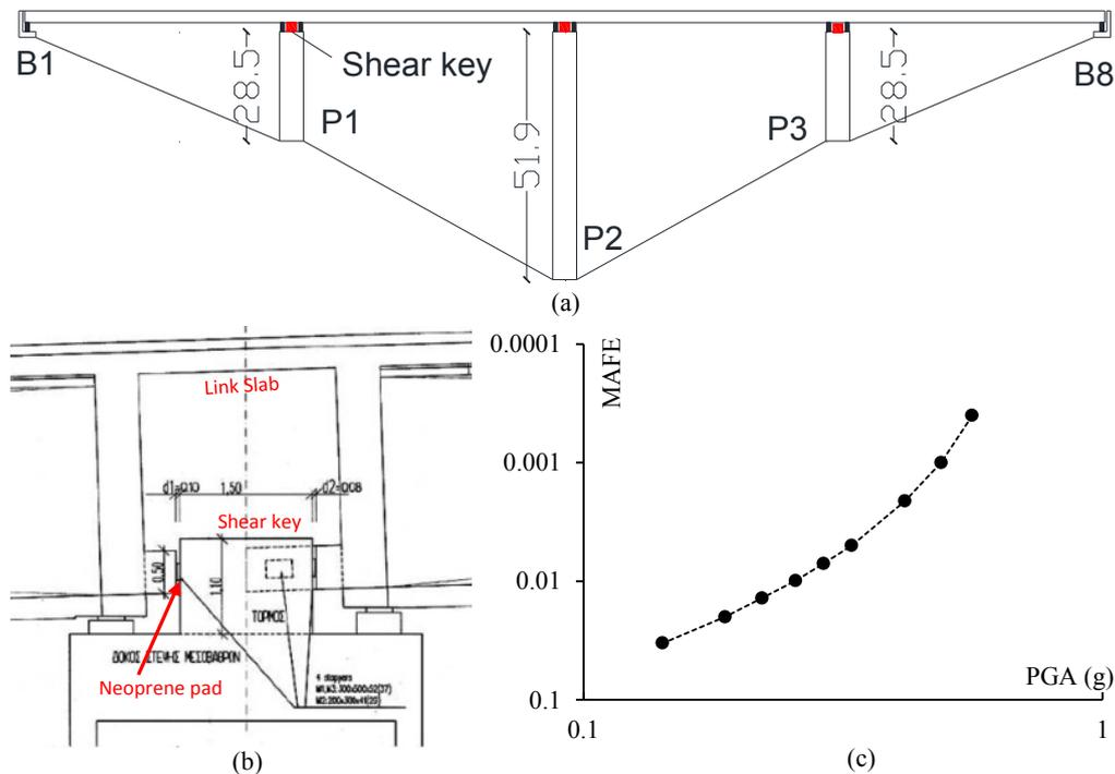
Figure 3: The 2nd Kavala bridge of the Egnatia Motorway: (a) Schematic bridge layout, (b) Details of link slabs and shear keys (c) Hazard curve of the bridge site.
