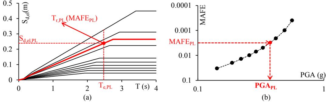
Figure 2: (a) Evaluation of the return period associated with the performance point of the structure, (b) Derivation of  $PGA_{PL}$  from the hazard curve of the bridge site.
