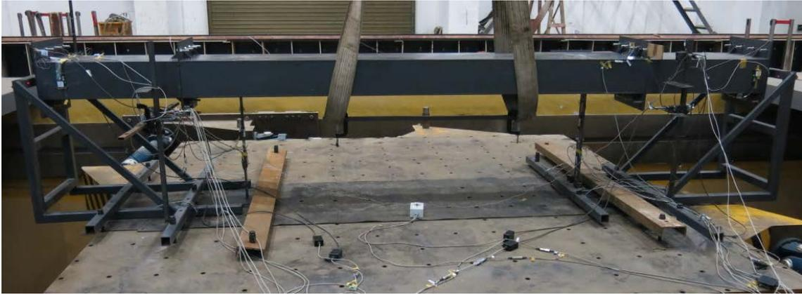
**Figure 1: Setup of straight bridge on shake table**
