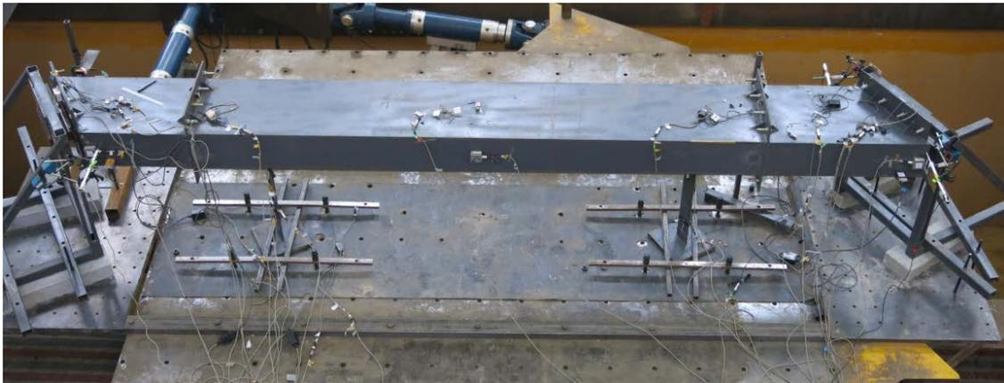
**Figure 2: Setup of 30° skewed bridge on shake table**
