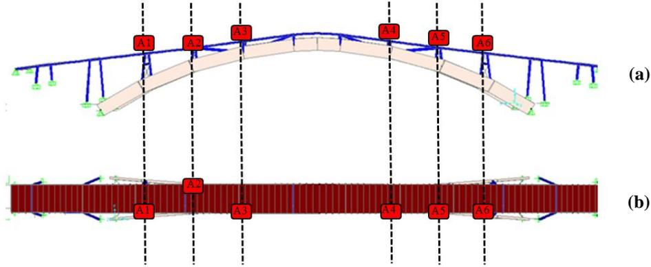
Figure 5: Position of the accelerometers. (a) Lateral view, and (b) Plane view.
