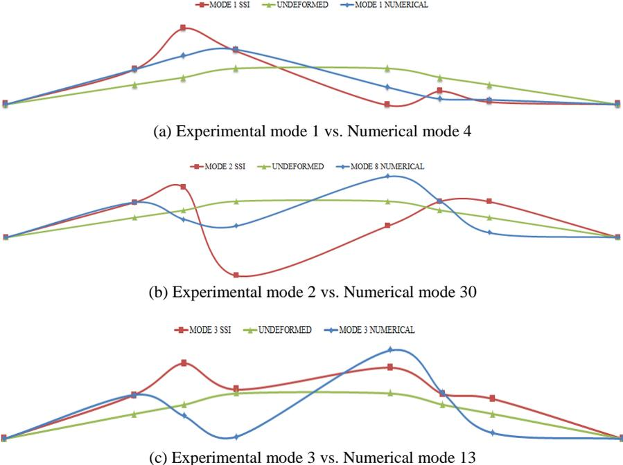
**Figure 9: Comparison of experimental and numerical mode shapes**
