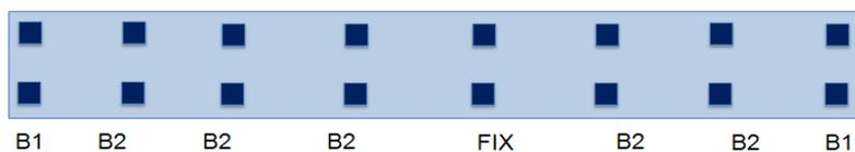
Figure 3: The bearing locations and numberings (plan view)
