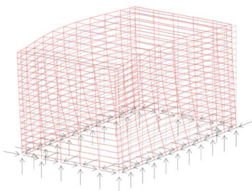
Figure 3: The Microstran analysis showing the first mode response, calculated as 8.6 Hz; the lowest racking mode in the orthogonal direction was at 16.2 Hz.
