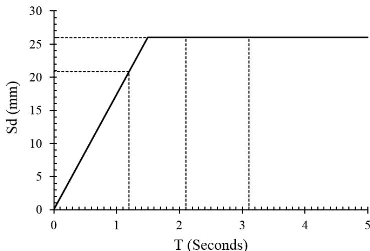
Figure 3: Elastic displacement response spectra
