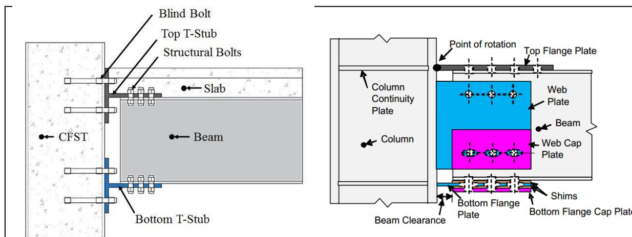
Figure 4: T-stub connection to CFST
