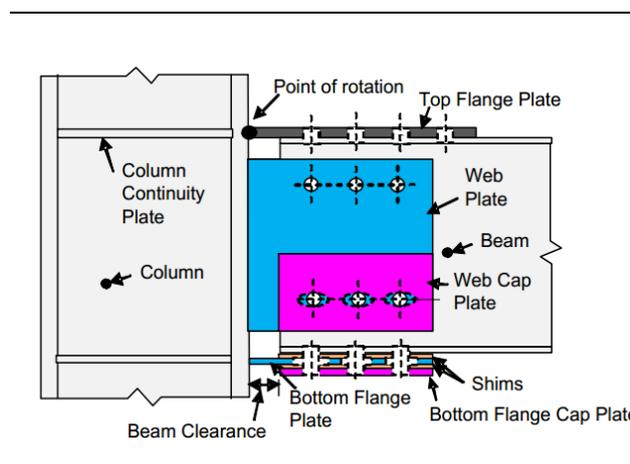
Figure 5: Sliding hinge joint (MacRae et al. 2010)
