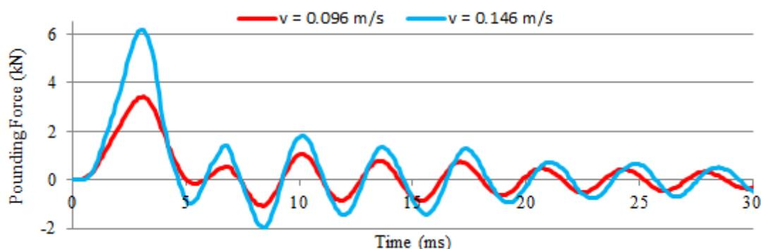
Fig. 6. Pounding force recorded from two impacts
