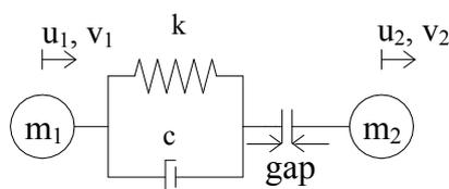
Fig. 3. Viscoelastic model of lumped mass impact.
