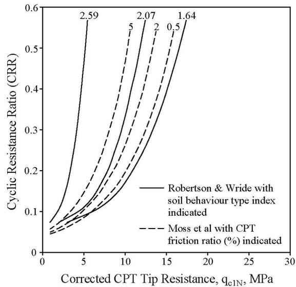
Figure 1: Comparison of Robertson & Wride (1998) and Moss et al (2006) liquefaction boundary curves for granular soils
