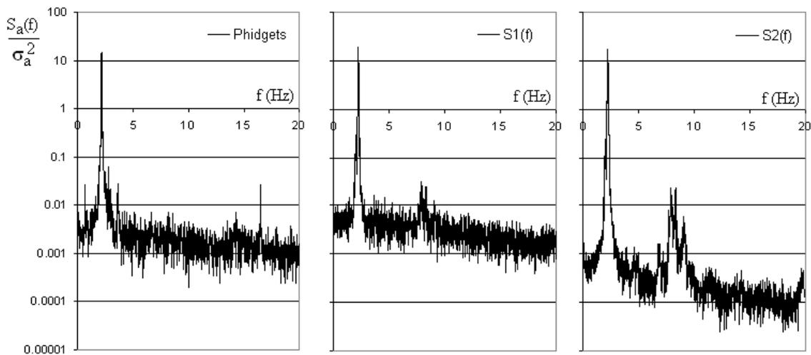
Fig. 7: Comparison of normalized acceleration response spectra Bridge#1
