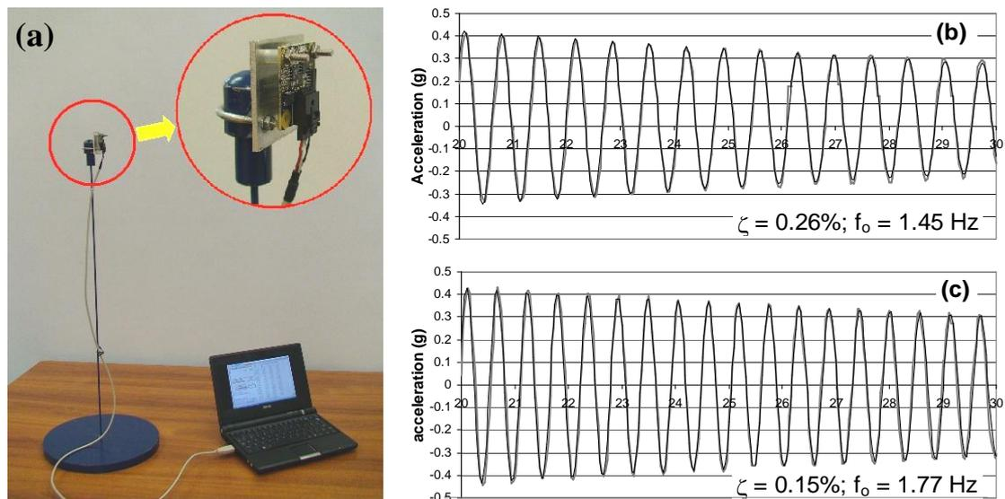
Fig. 3: Experimental investigation of a vertical cantilever using a Phidget accelerometer
