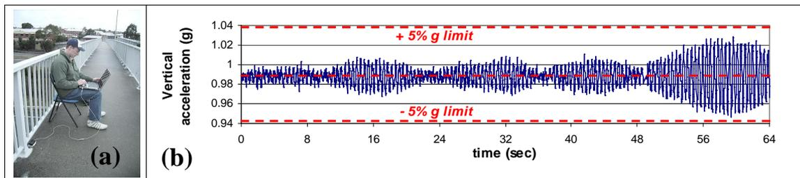
Fig. 4: Single pedestrian excursion of Bridge#1 (a) Sampling (b) Example trace
