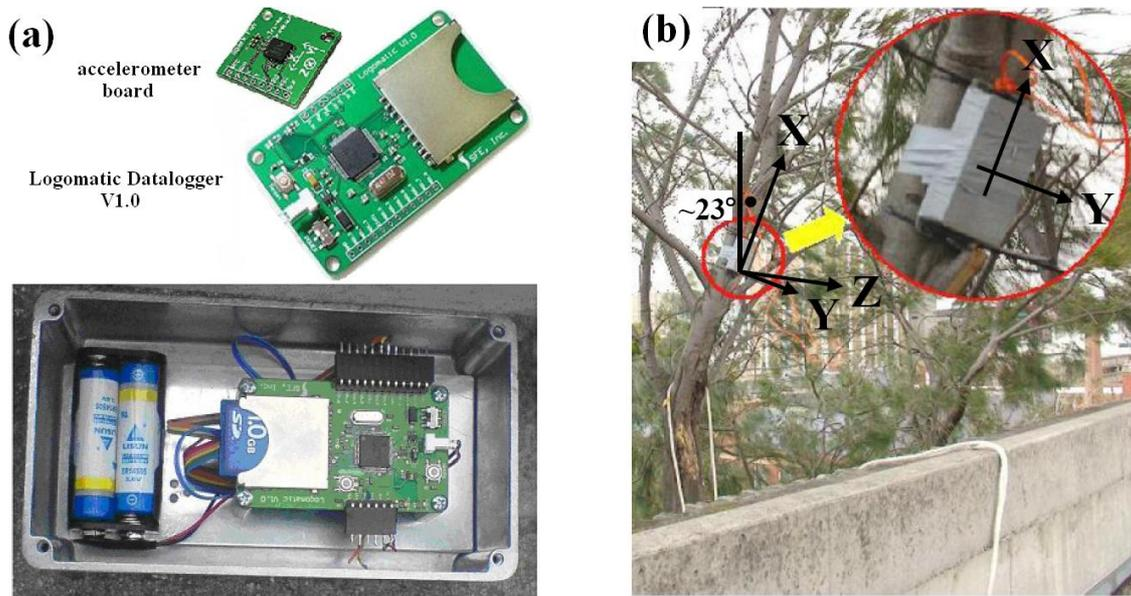
Fig. 5: (a) Logomatic data-logger accelerometer system pack (b) Pack mounted on tree
