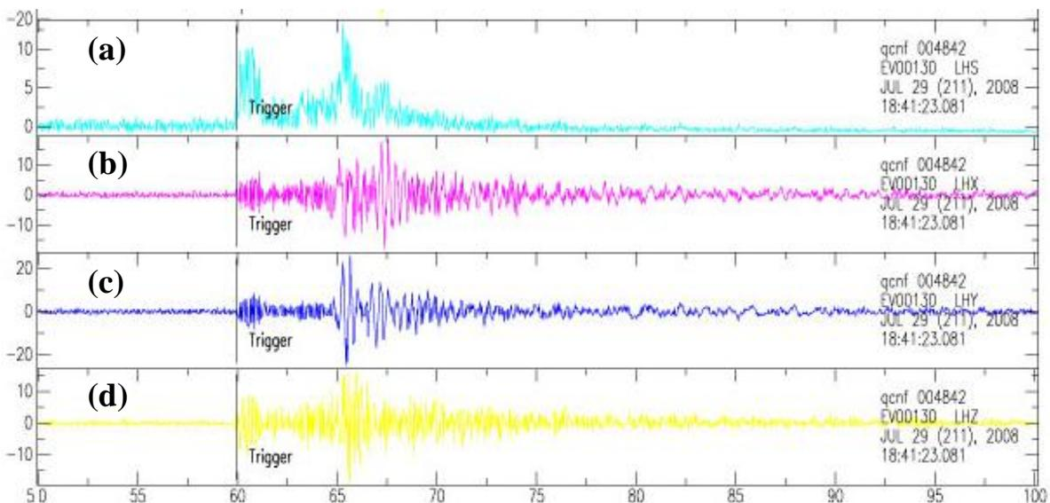
Fig. 2: QCN site vibration records: (a) significance filter (current shaking compared to shaking in the past minute); (b) left to right (not oriented geographically); (c) front to back; (d) vertical motion (Source: <http://qcn.stanford.edu/earthquakes/2008/211/> )
