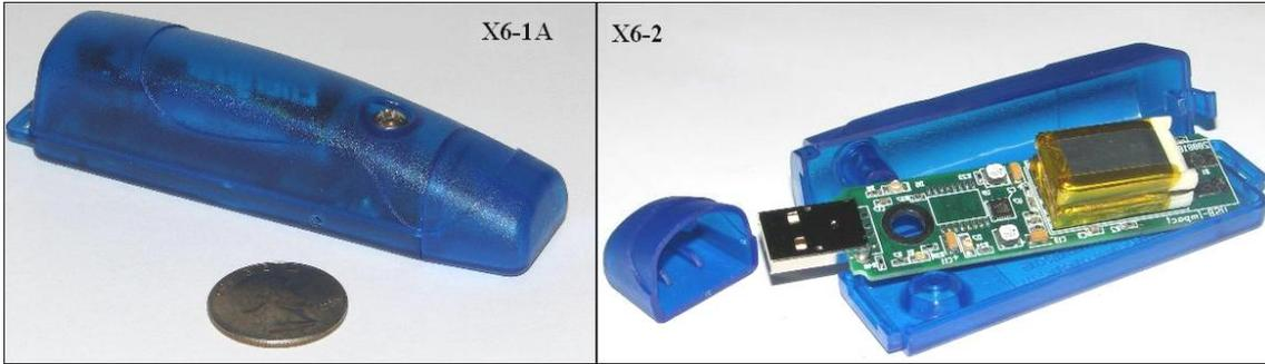
Fig 6: View of GCDC MEMS based accelerometer data-loggers X6-1A and X6-2
