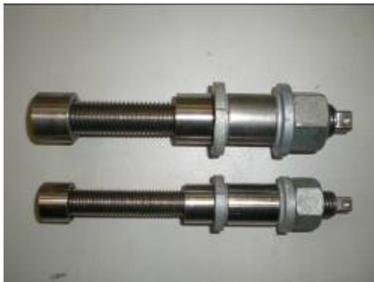
Figure 1 Modified blind bolts with extensions
