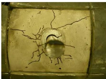
**Figure 9 Concrete in specimen T6\_D20\_N2**
