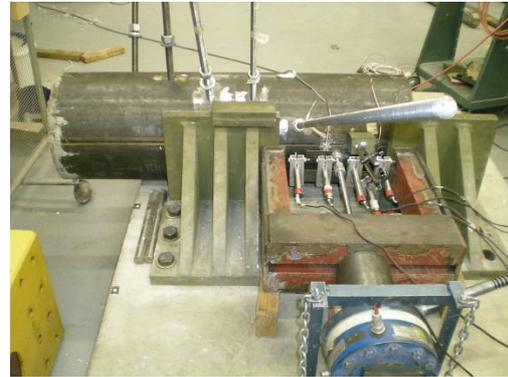
Figure 4 Setup of pullout test on CHS column
