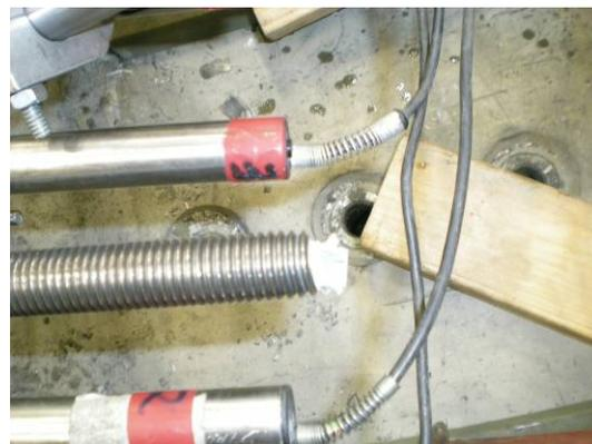
**Figure 7 Tube wall yield & bar pullout**
