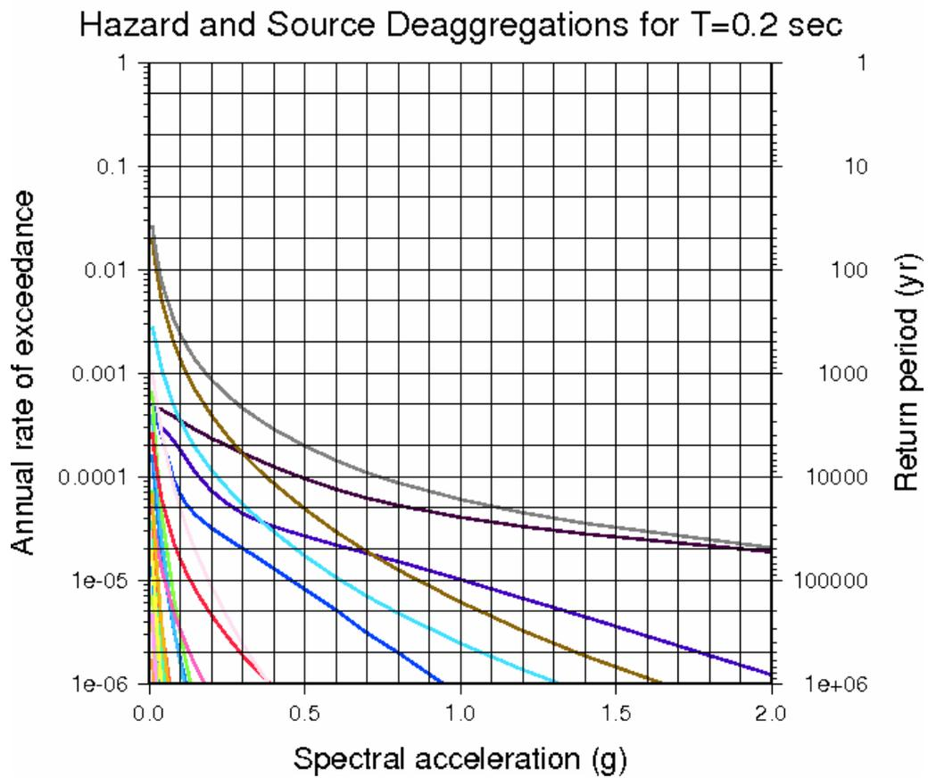
Figure 2. Disaggregation of the hazard curve by faults and source zones for spectral acceleration at 0.2 seconds period.
