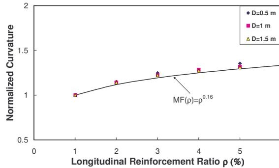
Figure 7: Influence of the Longitudinal Reinforcement Ratio
