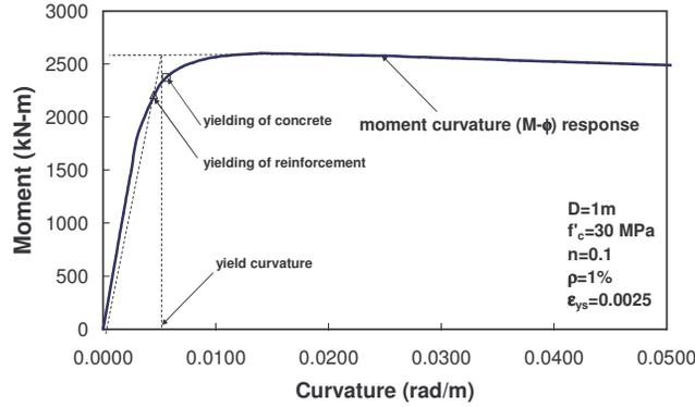
Figure 2: Moment curvature ( $M-\phi$ ) response
