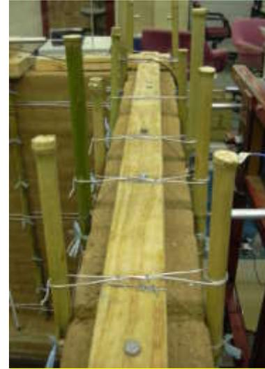
Figure 2b. 3J: Connection between bamboo + ring beam.
