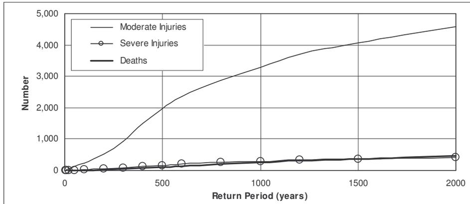
**Figure 2:** Estimated numbers of deaths and injuries in New Zealand earthquakes as a function of return period. Numbers of critical injuries were too small to plot. In all cases “Number” is the number that was equalled or exceeded for the given return period.
