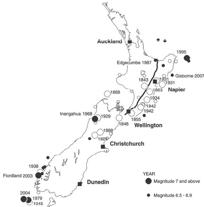
**Figure 1:** Occurrence of moderate-large shallow earthquakes in New Zealand since 1840. Filled circles are for recent earthquakes, 1955 to 2007 inclusive, and open circles for pre-1955 events. The Wellington Fault and associated structures are shown as a heavy black line.
